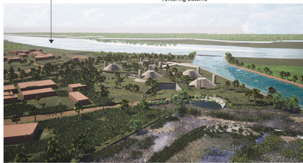
TERRACED BIOSWALE Water physical filtration on each terrace by bioswale system before entering cisterns
